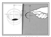
Around drain pipes, fold the sheet against the pipe and mark a line on the material where the center if the pipe is. Cut a hole about 25 mm (about 1 in.) smaller than the diameter of the pipe. As shown, cut the hole at the start of the fold. Heat the sheet vinyl and press it over the pipe. trim off excess material with o hook knife so that the break in the pipe wall is cleared.
