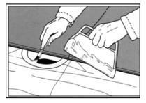
Fold back and loosen the sheets covering half of the floor area.
