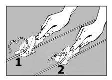
CAUTION: Welded seams must cool to room temperature before trimming. Start trimming where you began welding. All trimming of welding rod is recommended in two steps: rough and fine trimming.
