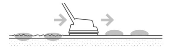
Small surface abrasions from traffic allow stains to penetrate and become embedded
